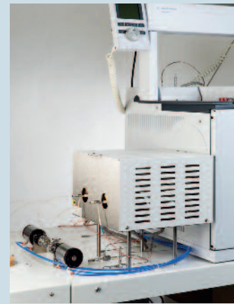
Nu GC-IRMS interface attached to the Agilent 7890 GC
