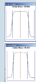
Automatic peak centre on N_2 and CO_2
