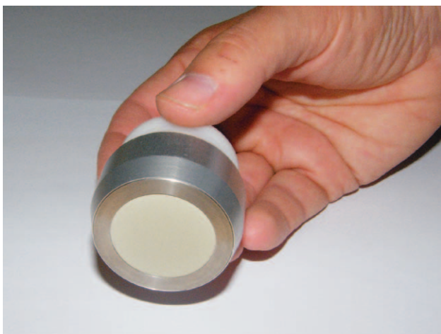
Figure 3. Standard 40 mm sample holder with cement pellet in place.
