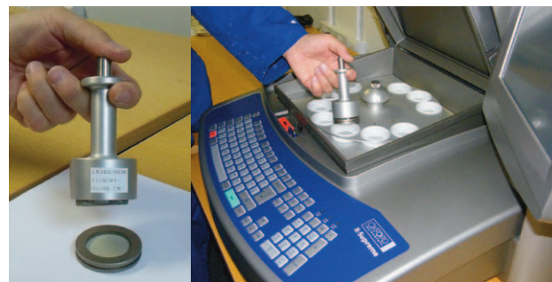
Figure 4. Pressed cement pellets in 51.5 mm (2 in.) steel rings are loaded into the magnetic holder and placed onto the 10-position sample carousel of the X-Supreme8000 instrument.
