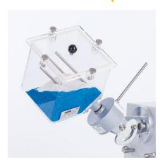
The Cube Mixer uses a tumbling motion to produce a homogenous blend within a short time. The mixing action is assisted by three stainless steel rods positioned inside the cube. The device is attached to the drive unit via the ERWEKA Universal Gear UG, which permits operation at various angles for optimal efficiency. Our cube mixers are avilable in the following versions:
