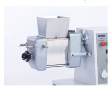
Wet granulator with oscillating rotor for the production of wet granules.
