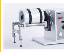
The Ball Mill is used for grinding crystalline materials and for mixing dry, or under certain circumstances, moist materials. The drum is available with 0.5, 5 or 10 l volume.
