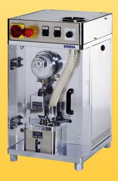
The EP-1 is the ideal desktop tablet press for R&D purposes. The single punch eccentric Tablet Press EP-1 can manufacture tablets and odd shaped products with a diameter of up to 20mm. It operates automatically i.e. the die is filled with powder or granule, the material compressed and the tablet ejected continuously.
