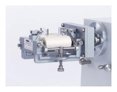
The three roller mill is used for the production of ointments, pastes, creams and similar products.
