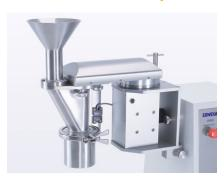
The CM is designed for homogenization of dry products to a specified particle size, reduction of oversized particles to the desired size and milling of agglomerates back to the initial size. A set of shims to adjust the clearance between the rotor and screen (0.5 mm to 3.0 mm) is supplied. It allows a flow rate of up to max 40 kg/h with a rotor speed of 0 - 1200 rpm. An safety interlock helps to prevent injuries.
