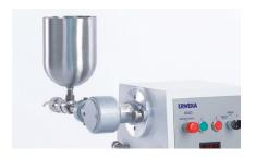
The homogeniser is used for homogenising fluids, both oil-in-water or water-in-oil emulsions. The media is filled into the upper bowl. Then a stainless steel piston presses the injected fluids through a ring nozzle into a valve, therefore homogenising the emulsion.
