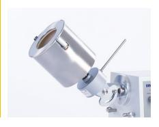
Polishing drum to polish coated tablets. The drum is covered with interchangeable felt parts.
