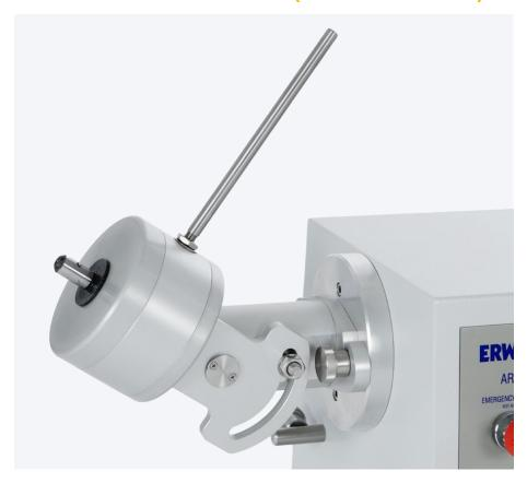
The new universal gear uses a modernised CNC machined aluminium design for improved durability. It is required for adjusting the angle of operation (0-80°) and reduction of speed (1:6).
