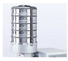
The Erweka VT operates on the reciprocating cam principle. The vibration intensity can be adjusted by changing the speed of the drive unit.
