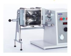
Laboratory kneader with stainless steel kneading vessel (5 liter volume, working capacity 65%) housing two z-shaped kneading blades running at different speeds in opposing directions.
