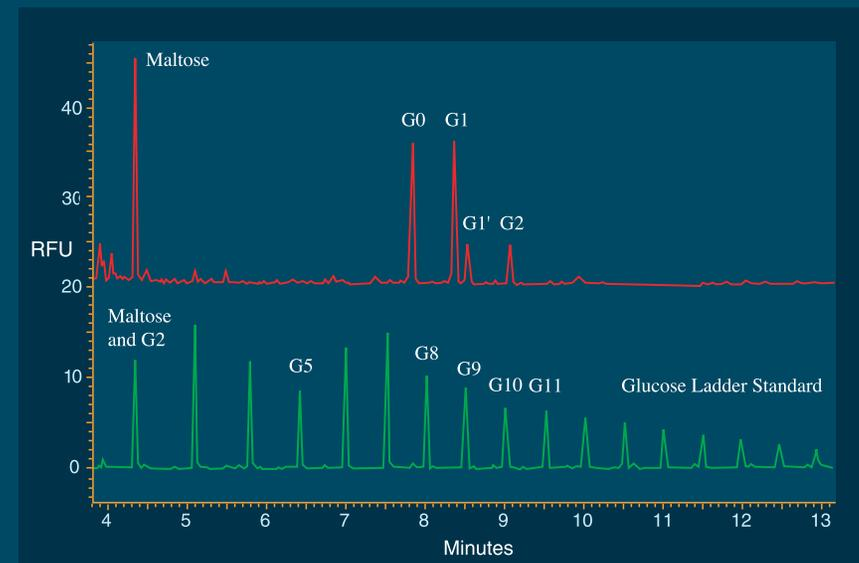
Oligosaccharide distribution associated with a protein yields a fingerprint that can be used in protein identification. The PA 800 Plus provides easy, quantitative and robust determination of protein microheterogeneity, with a typical analysis time of less than 15 minutes.
