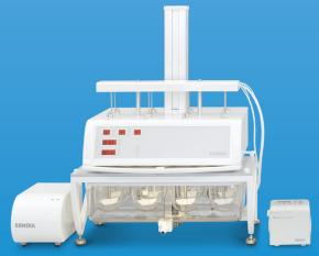
The online dissolution system consists of a DT 72x, an IPC 8 and connects UV/VIS spectrophotometer for online determination of dissolution rates. The system is managed by our Disso.net PC software
