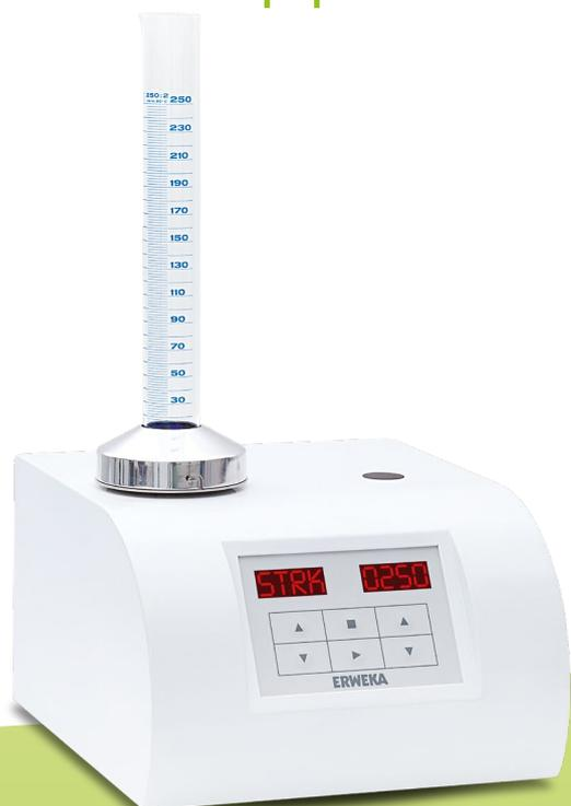
The ERWEKA SVM has been designed for measuring the tapped volume and tapped density of powders, granules and similar products.
