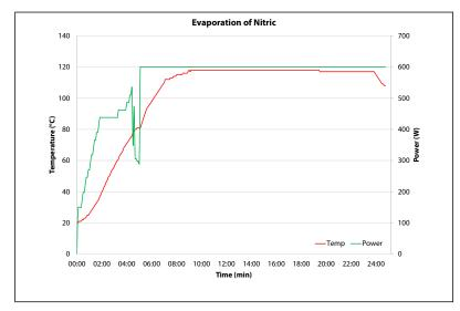
In the post concentration step the Plateau was detected at 117° C. The system continued to run until the temperature dropped by 10° C. Preconcentration, digestion, and evaporation of all samples was done in the same liner eliminating loss or cross contamination due to sample transfer.
