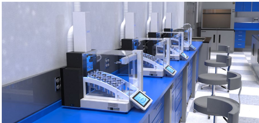
Figure 1: High throughput analysis of 48 samples/hr with four Energized Dispersive Guide Extraction (EDGE) systems.
