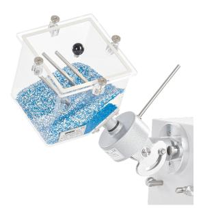
The Cube Mixer uses a tumbling motion to produce a homogenous blend within a short time. The mixing action is assisted by three stainless steel rods positioned inside the cube. The device is attached to the drive unit via the ERWEKA Universal Gear UG, which permits operation at various angles for optimal efficiency. Our cube mixers are available in the following versions:
