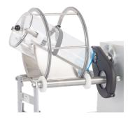
Drum Hoop Mixer with diagonal placement of the drum within the hoop, available with 5 and 10 liter volumes. The rotation of the hoop itself produces a uniform, three-dimensional displacement of the material to be processed and hence a tumbling mixing action.
