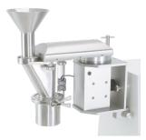
The CM is designed for homogenization of dry products to a specified particle size, reduction of oversized particles to the desired size and milling of agglomerates back to the initial size. A set of shims to adjust the clearance between the rotor and screen (0.5 mm to 3.0 mm) is supplied. It allows a flow rate of up to max 40 kg/h with a rotor speed of 0 - 1200 rpm. A safety interlock helps to prevent injuries.
