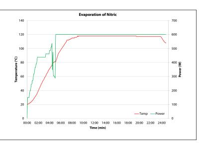
In the post concentration step the Plateau was detected at 117° C. The system continued to run until the temperature dropped by 10° C. Preconcentration, digestion, and evaporation of all samples was done in the same liner eliminating loss or cross contamination due to sample transfer.
