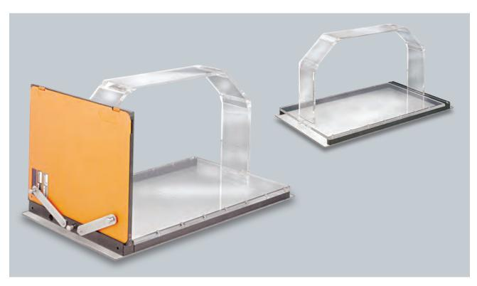
Together with features embedded in our BrachyVision™ treatment planning software, the Reconstruction Jigs may be used to create brachytherapy treatment plans from semi-orthogonal films such as those obtained with the use of a C-Arm. The jigs are made of acrylic and aluminum. They incorporate horizontal and vertical film holders, and embedded fiducial markers used by the planning software to create a common coordinate system. Two sizes are provided to accommodate a range of patients.
