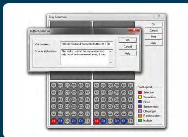
Figure 8: Buffer trays may be annotated with full descriptions – including buffer preparation protocols and saved as part of the method.
