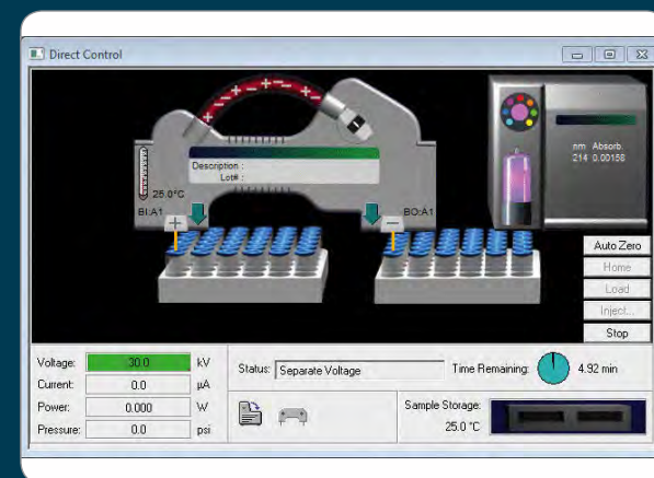
Figure 9: Direct Control – A graphical interface to select and change operating parameters with immediate real time execution and status display.
