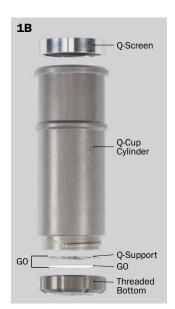
**Figure 1.** Positioning of the G1 and C9 Q-Discs, used in the extraction of the non-hydrolyzed samples (**A**) and the positioning of the Q-Support and G0 Q-Disc, a combination called G0 used in the extraction of the hydrolyzed samples (**B**).
