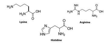
CEM's proprietary iTag solution binds to these three amino acids using an acid group. The aromatic portion of the molecule absorbs light and is easily detected with a colorimeter.
