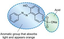
A pre-determined amount of iTag solution is added to a sample and homogenized to release the proteins. The iTag molecules bind to the proteins and are removed from solution. The remaining iTag is drawn up through a disposable filter into the built-in colorimeter. The amount of iTag bound to the protein is determined and the results displayed. The entire process takes only 2 to 3 minutes for most samples and yields results that are more accurate than Kjeldahl or combustion techniques.
