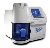
Protein is also directly tested using the **Sprint** Rapid Protein Analyzer, eliminating calibrations and drifting results, using dye-binding technology. CEM's proprietary iTag Solution binds directly to protein molecules at 4 distinct locations, ensuring only true protein is read. Other technologies use nitrogen analysis, which can produce inaccurate data as a result of adulterants or miscalculations.
