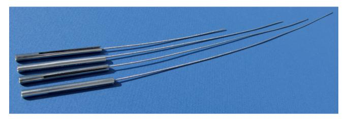
Length cutting gauges allow for catheters and implant tubes to be cut to one of several exact lengths (113 mm, 200 mm, 250 mm, 320 mm, and 500 mm) so that the applicator/source guide tube combination length is 1300 mm.
