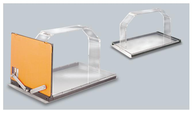
Together with features embedded in our BrachyVision™ treatment planning software, the Reconstruction Jigs may be used to create brachytherapy treatment plans from semi-orthogonal films such as those obtained with the use of a C-Arm. The jigs are made of acrylic and aluminum. They incorporate horizontal and vertical film holders, and embedded fiducial markers used by the planning software to create a common coordinate system. Two sizes are provided to accommodate a range of patients.
