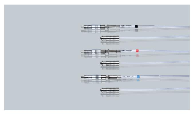
The GammaMed*plus* source guide tubes with locking mechanism and the PDR quick connectors enable easy, safe connection of applicator probes, needles and interstitial implant tubes to the afterloader. The source cable is blocked in case of an improper connection at the applicator end. An error message is also generated in case of an improper connection at the afterloader end.
