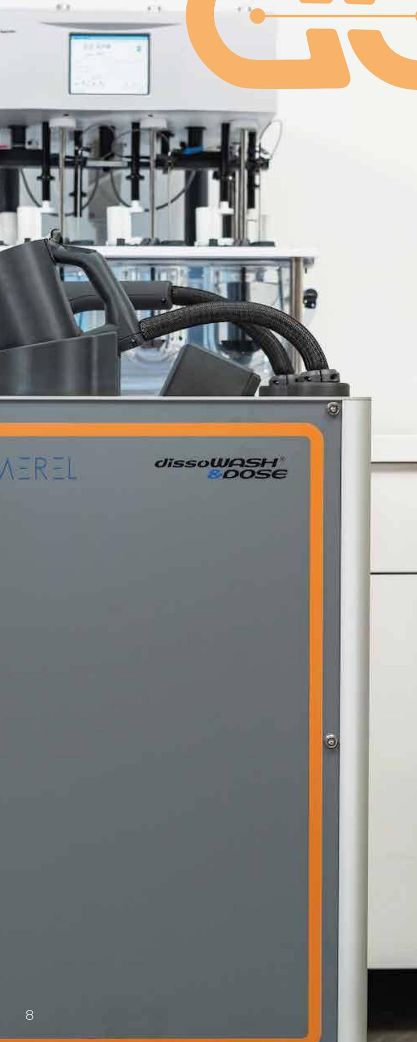
One of a kind, semi-automated and easy to use dissolution tester washing system with media dispensing capability. Battery powered for superb mobility and fully equipped for exceptional performance.
