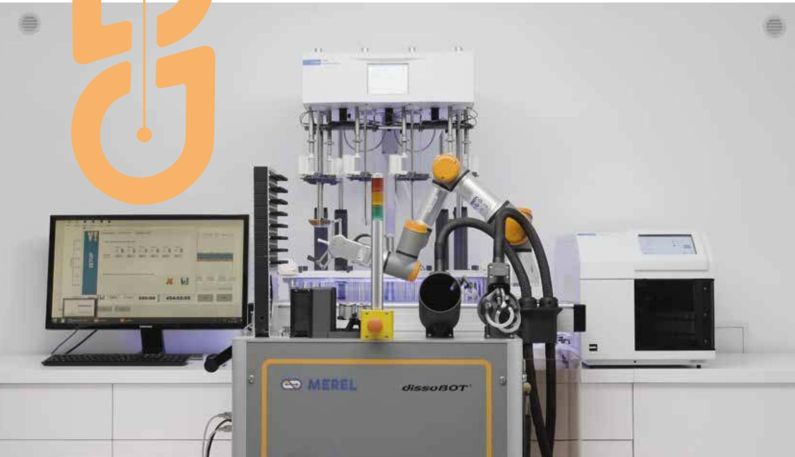
The world's first fully automated dissolution system with clip-on/off capability.
